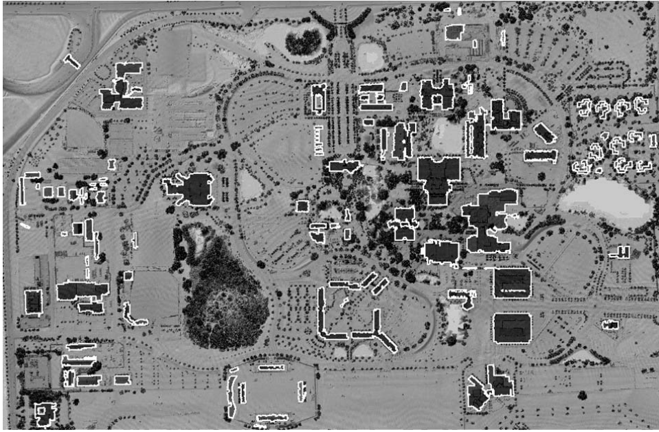
Fig. 6. The raw footprints for buildings at FIU Campus. Raw footprints were derived by connecting boundary points of identified building measurements using the region growing algorithm. The background image was derived by interpolating raw LIDAR point measurements.
