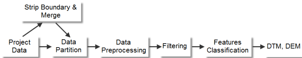
Figure 7-1 Schematic procedures for LIDAR data processing
