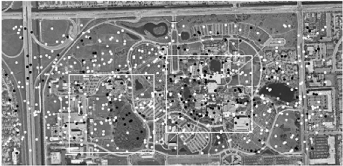
Figure 12: Aerial photograph for the University Park campus of Florida International University. 648 random sample points are also overlain over the photograph. The ground and non-ground measurements identified from these samples by the progressive morphological filter are represented by white and black dots, respectively. The white rectangles represent the range of Figure 13 and 14
