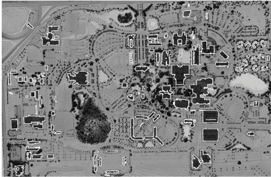
Figure 31: The raw footprints for buildings at FIU Campus. Raw footprints were derived by connecting boundary points of identified building measurements using the region growing algorithm. The background image was derived by interpolating raw LIDAR point measurements.
