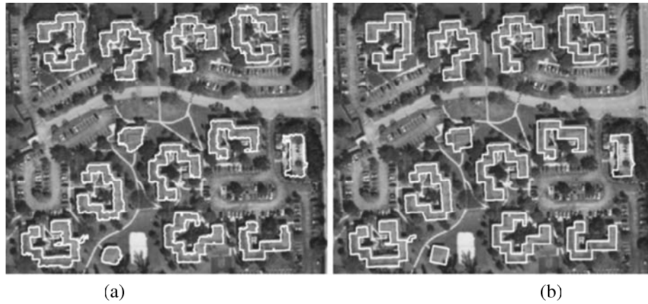
Figure 33: Comparison of raw (a) and adjusted (b) building footprints. The small "zig-zag" noise in the raw footprints was removed in the adjusted footprints, making the adjusted footprints look more realistic.
