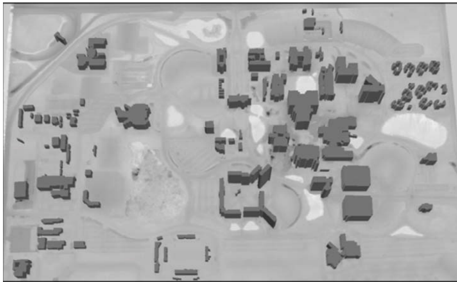
Figure 35: 3D building models for FIU campus. Each building model was created using the final footprint and average building height derived from LIDAR measurements. The DTM for building bases was derived by interpolating ground measurements identified by the progressive morphological filter.
