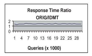
Fig. 8. Response time ratio of the server with the original thread pool model and the server with the IDMT model, in the case of that one client sends continuous requests.
