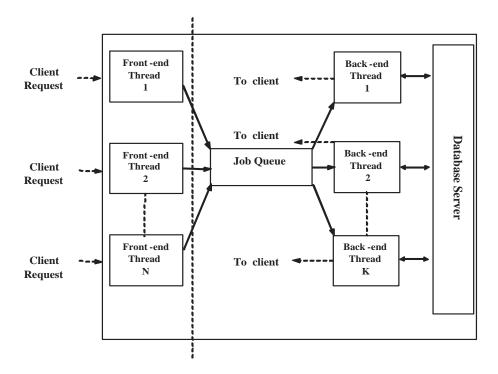
Fig. 4. The Internally Distributed Multithreading (IDMT) model design.
