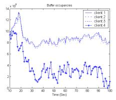
Figure 3. Buffer Occupancies when only client 4 uses adaptive playback.
